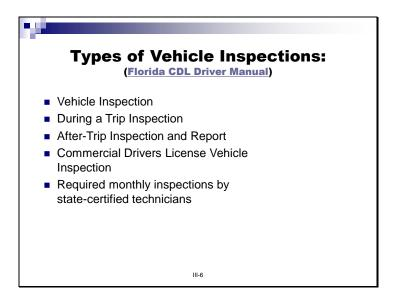
There are five basic vehicle inspections. The operator conducts four of these inspections.
