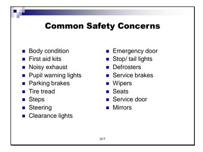
The following areas should be looked at during vehicle inspections because defects can lead to unsafe conditions.
